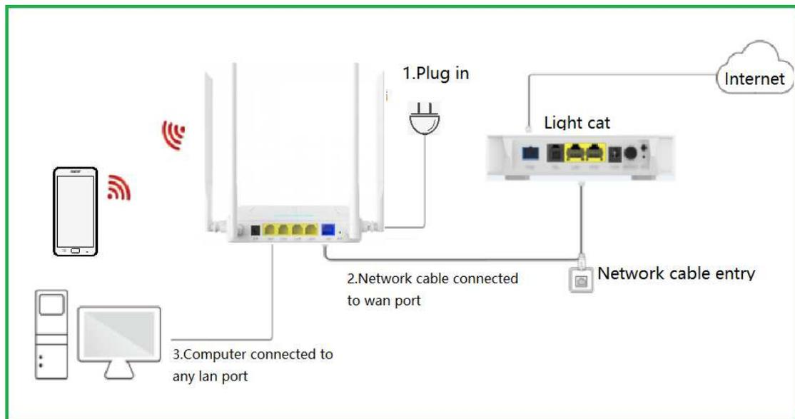
Note: When the WAN port or LAN port of the router is plugged into the network cable, the corresponding indicator will flash. If there is no response when the network cable is inserted, please check the network cable and the corresponding interface.
