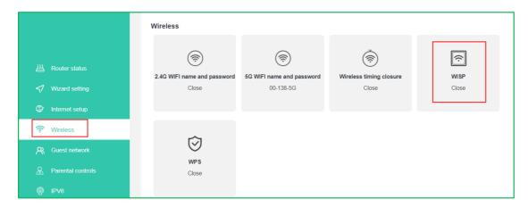
3.Turn on the WISP, select the mode "WISP" or "Repeater (Client+AP)", and then click the refresh icon behind the wireless network selection. After scanning the signal, select the relay wireless signal.
