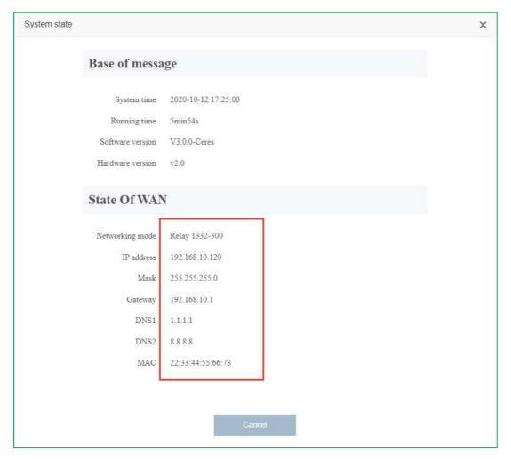
**Note:** If you use the Repeater (Client+AP) mode, after the relay is completed, the IP of the router is issued by the superior. At this time, if you want to login to the management interface of WR133F, you need to set a static IP on the computer. The operation is as follows:
