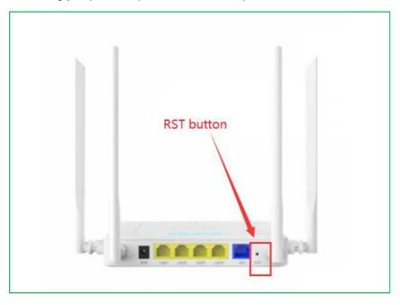
2. Wait for a minute around, when the WIFI indicator lights up again, open the browser, input the management IP(refer to the sticker at the bottom of the router)or "www.ceres.com" in the address bar, click the Enter key to enter to the login page, the factory login password is admin (refer to the sticker at the bottom of the router), click login to enter the management page. After logging in, the following interface will appear, proving that the factory settings are restored successfully.
