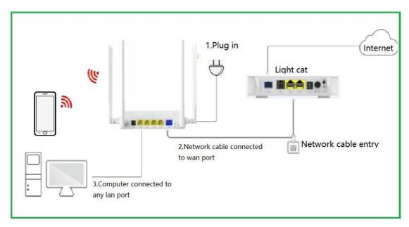
Note: When the WAN port or LAN port of the router is plugged into the network cable, the corresponding indicator will flash. If there is no response when the network cable is inserted, please check the network cable and the corresponding interface.
