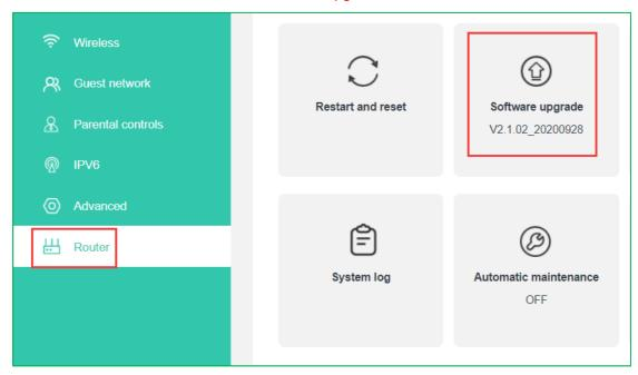
3.Enter the software upgrade interface, click "Upgrade", click "Choose File", a way to select files will pop up, select the file to be upgraded, click OK, the upgrade interface displays the name of the new software version, click OK to upload. (Note: The upgraded file format is bin format)
