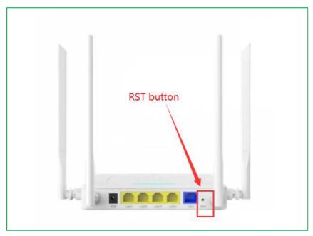
2. Wait for a minute around, when the WIFI indicator lights up again, open the browser, input the management IP(refer to the sticker at the bottom of the router)or "www.ceres.com" in the address bar, click the Enter key to enter to the login page, the factory login password is admin (refer to the sticker at the bottom of the router), click login to enter the management page. After logging in, the following interface will appear, proving that the factory settings are restored successfully.
