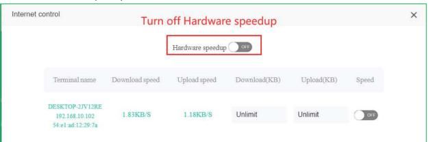
3. Find the device that needs to be restricted, as shown in the figure below, open the speed limit icon on the right, fill in the speed limit flow, fill in 1024 in the upstream, and then click on the blank area of the interface to take effect. (Internet speed limit only needs to enter numbers, no need to enter units)
