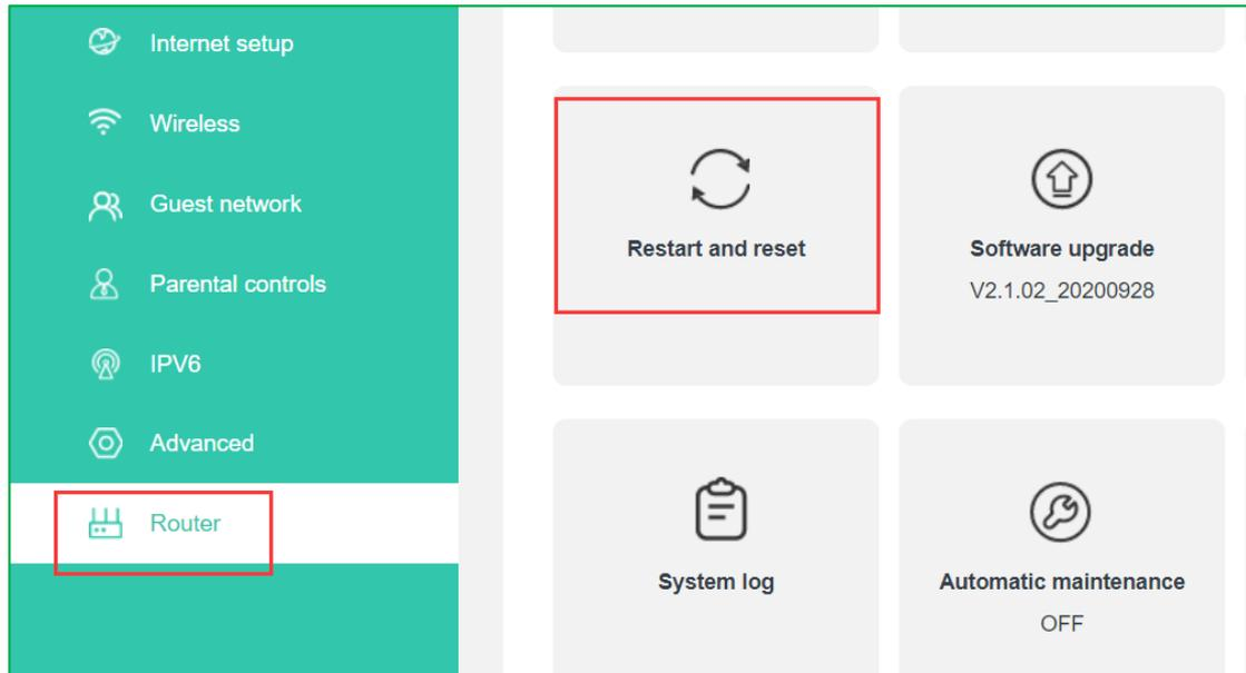
3. Click the "Reset" button on the right to restore factory settings. A pop-up window appears, then click "Confirm" to display the reset progress bar. After resetting successfully, it will jump back to the login interface so that all the router settings will be restored to the factory settings.
