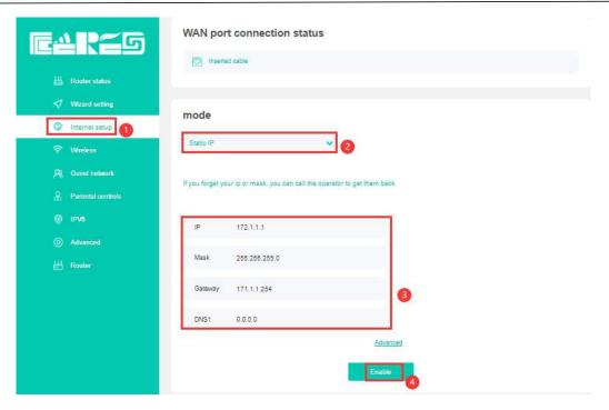
After finshed all of the configuration, click 'Enable' button to finish "Static IP" setting.
