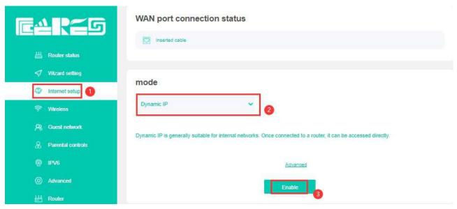
After finshed all of the configuration, click 'Enable' button to finish "DHCP" setting.
